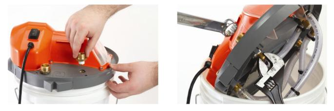
Thread male garden hose connector into opening marked "Chemical In" and tighten using two wrenches one on the fitting and the other on the brass elbow on the underside of the lid.
