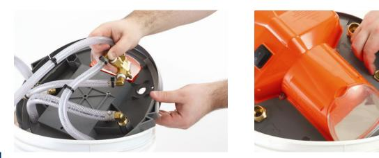
Loosen set screw in valve handle and remove handle and fastening nut; insert valve in opening marked "Chemical Valve" from the underside of the lid as shown and replace fastening nut to secure onto lid. Replace valve handle and tighten set screw to secure handle to valve.
