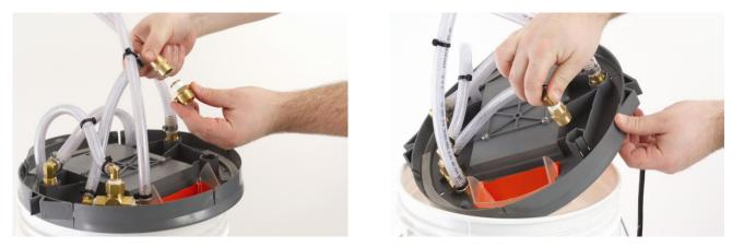
Remove male garden hose connector from valve assembly and insert female fitting into the opening marked "Chemical In" from the underside of the lid.
