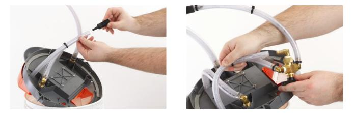
Detach black inlet strainer by cutting the clamp in place and removing the strainer from inlet tube. Press tube onto center barb of flow control valve; fasten in place with black tie wrap.
