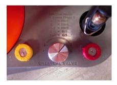
\*If an external water source is unavailable, use the remaining water in the CoilJet's water tank to fill the chemical tank. First, turn the chemical mixing valve clockwise (as many rotations as it takes) to the 'O' closed position. Do not over-tighten! Next, using the spray gun without a nozzle attached, fill the chemical tank with water. You will need to have about 2/3 of the water tank full for this flushing procedure.
